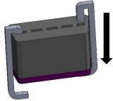
Pull the hooks into the holes of the OBD socket jack
